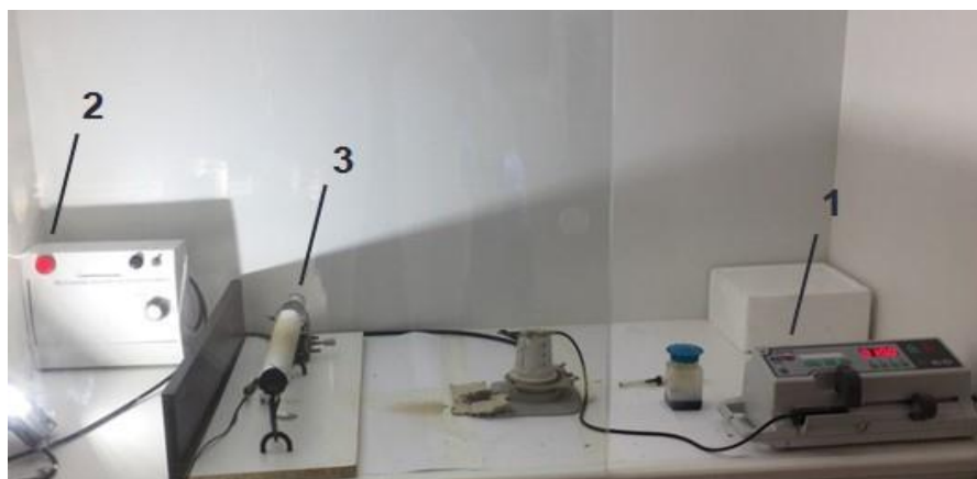
Figure 2 – Laboratory installation of electrospinnagug: pump syringe (1), high-voltage power source (2), substrate of aluminum foil (3)
